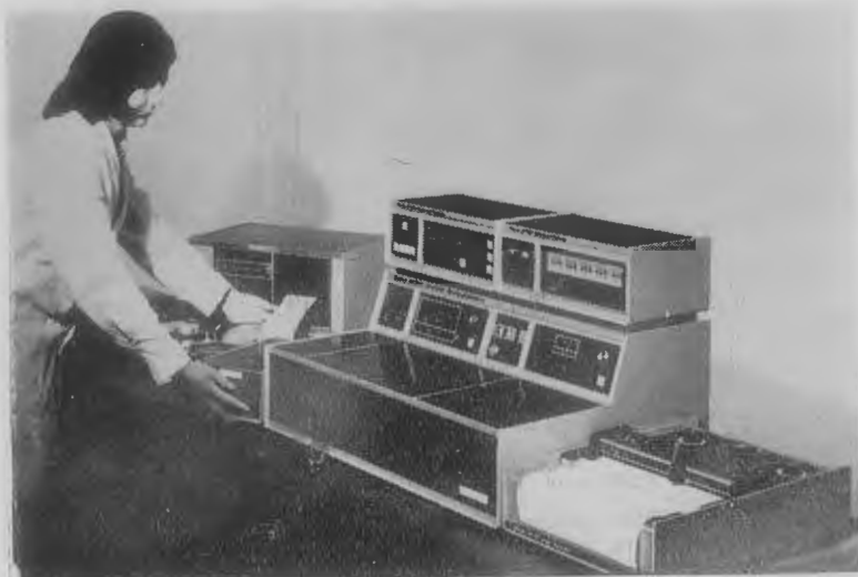
Fig. 1 The new Unicam SP8000 ultraviolet spectrophotometer made by Pye Unicam Ltd. — shown here with SP40 automatic sample-changer (left front), SP46 digital printer (left rear), SP8005 programme controller (rear) and an external recorder (right) in addition to the built-in recorder.
